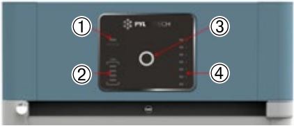
Fig. 2.4 - Control Module FC0500-40S-V2 Display Panel 1) System status, 2) System SOC (Each LED indicate 25% SOC), 3) LED button, 4) Battery Module Status
